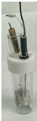
Figure S11. Photo of the three-electrode electrochemical cell used in the current work.
