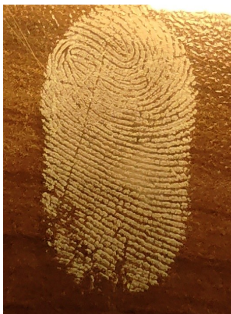
Figure S16 Bright-field image of LFP dusted with YOF: 0.01 Tb 3+ , 0.001 Eu 3+ nanophosphors captured under a fluorescent lamp.
