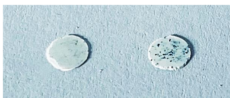
Fig. S1 Photograph of BG (left) and Ag@Cu-MOF@BG (right) discs.
