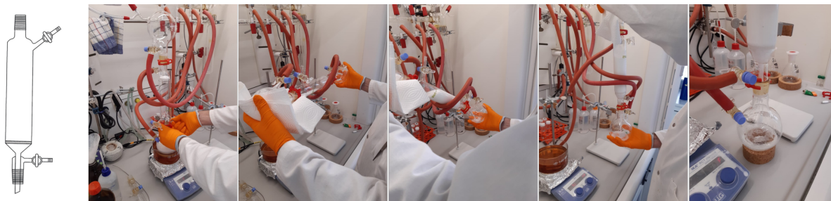
Figure S1: Schematic diagram of the reversible glass frit and pictures of the air- and moisture-free Schlenk filtration.
