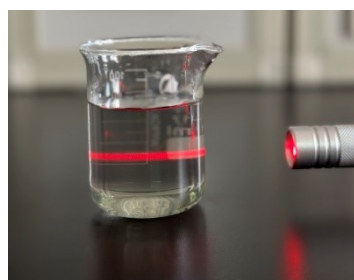
Fig. S1. (a,b) Tyndall effect of the MXene solution.
