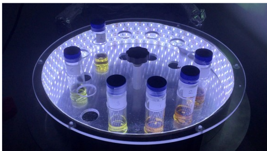
Figure S16. Photo of the photoreactor used for the photocatalytic experiments.
