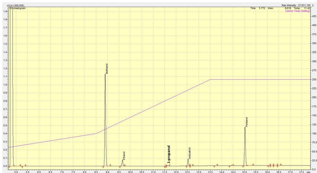
Figure S46. GC-FID chromatograph of methanol/ethanol upgrading reaction using catalyst 2 H ; pentanol is the internal standard.
