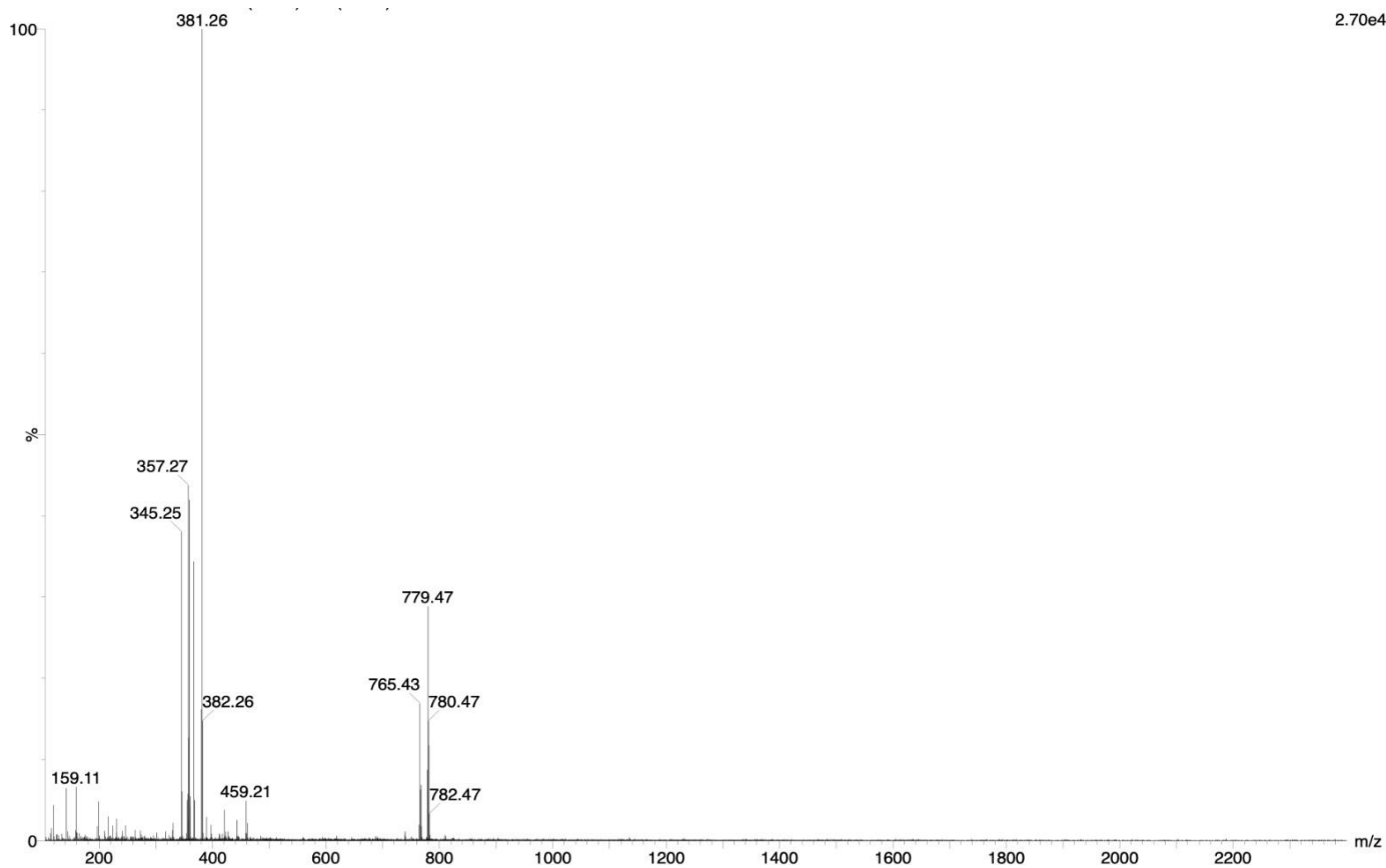
Figure S86. Mass spectrum of 2.BH3 in acetonitrile.
