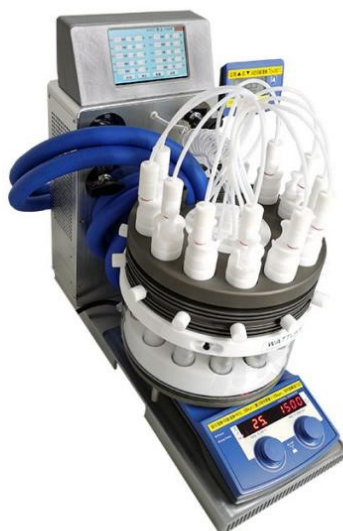
Fig. S1 Schematic view of WP-TEC-1020HSL of WATTCAS photoreactor instrument for photocatalytic measurements.
