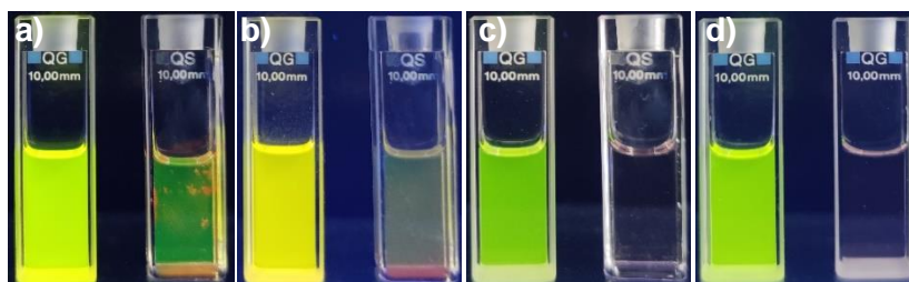
Fig. S4 Images of the emission ( \lambda_{\text{exc}} = 365 \text{ nm} ) from nonaggregated and aggregated samples of: (a) PDI1 in \text{CHCl}_3 (left) and hexane (right); (b) PDI2 in \text{CHCl}_3 (left) and hexane (right); (c) PDI-CB1 in dioxane (left) and water (right); (d) PDI-CB2 in dioxane (left) and water (right).
