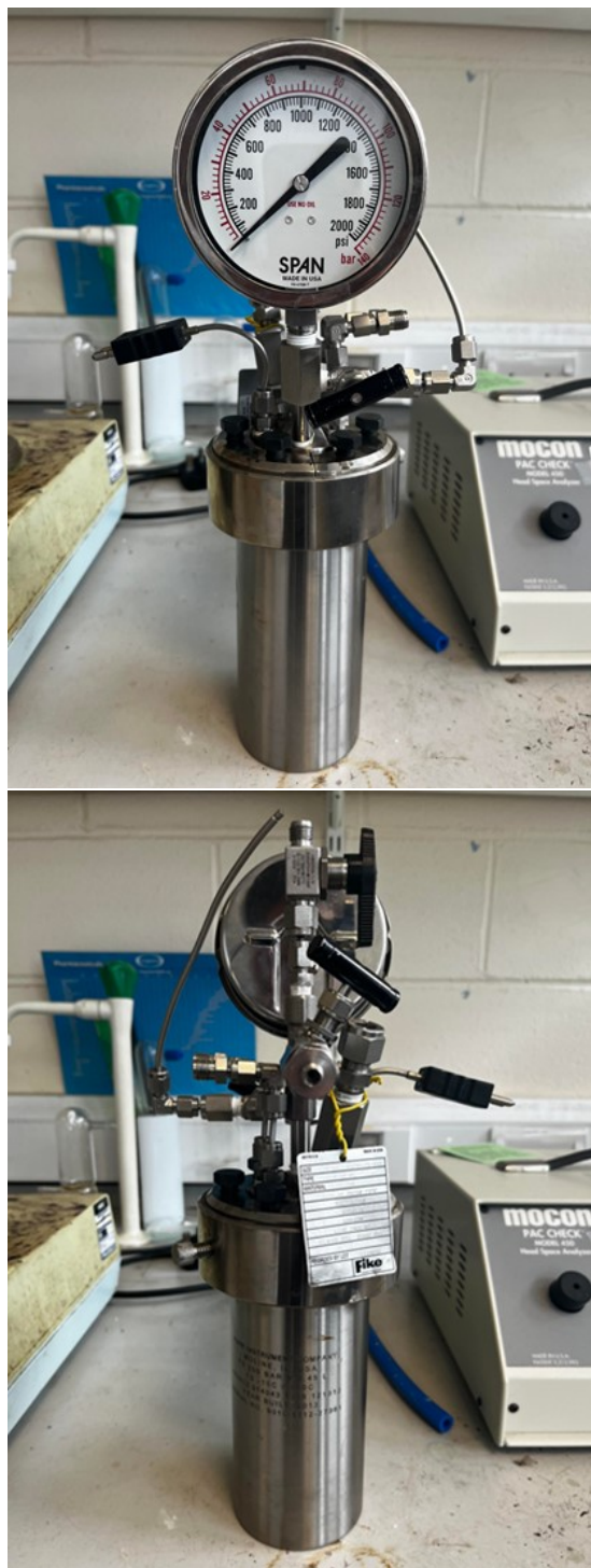
Figure S13. Stainless steel autoclave set-up for ROCoP of CHO/CO 2 , adapted for use with Schlenk line.
