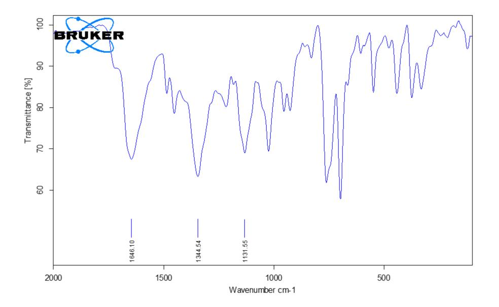
Figure S12. IR spectrum of Pt(DMSO)L(mal) (3)
