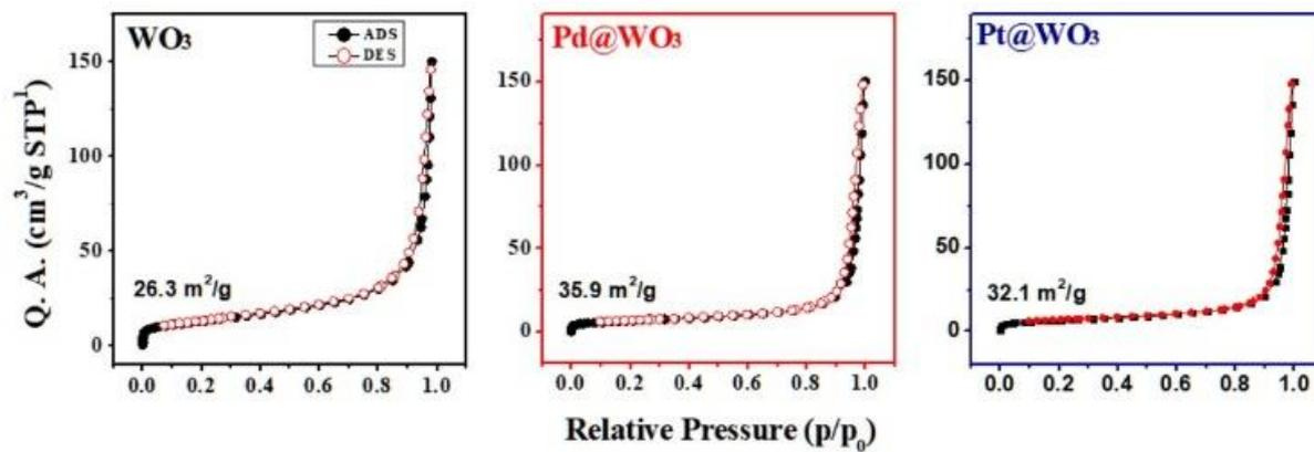
**Figure S2.** Brunauer–Emmett–Teller (BET) analysis of WO<sub>3</sub>, Pd@WO<sub>3</sub>, and Pt@WO<sub>3</sub> NPs.
