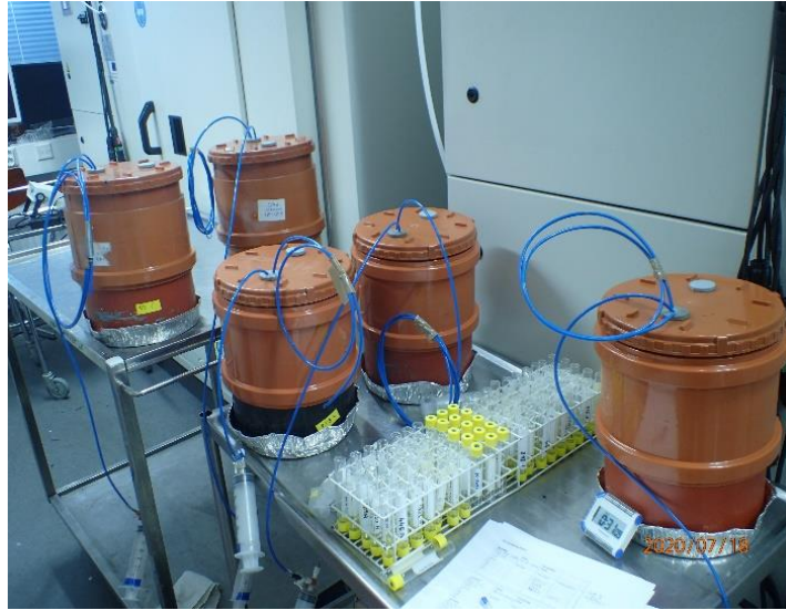
Fig. S1 CH 4 and N 2 O measurement set up in the laboratory using static dark chamber method. The chamber is positioned over the soil core and gas sampled from the chamber headspace with syringe into evacuated vials.
