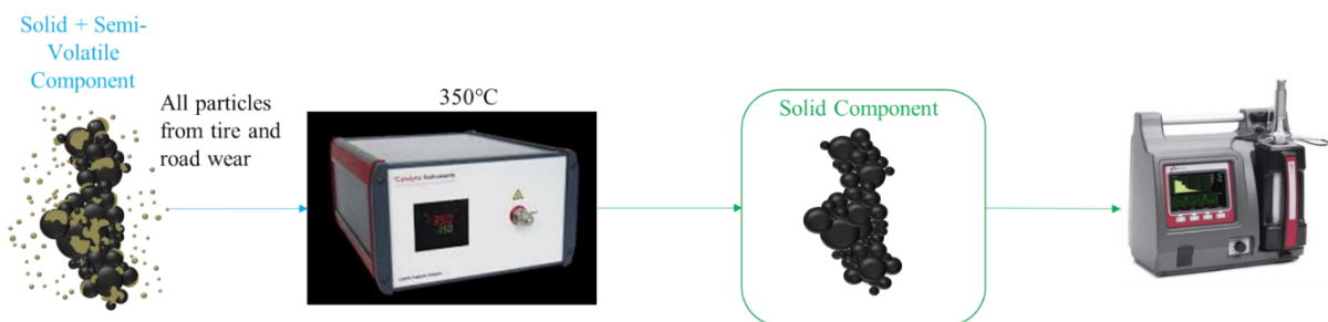
Figure S5. Sampling process shown for total particles (solid and semi-volatile particles) that go into the CS, with on the solid fraction coming out, which can then be sampled and sized/counted by the ELPI.
