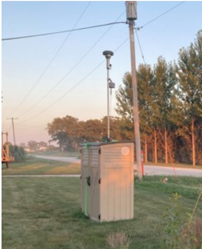
Fig. S4. The Site 1 sample shed containing a BAM monitor positioned near a rural unpaved road.
