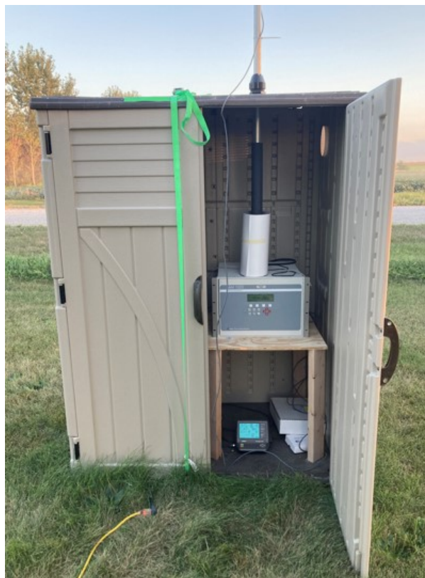
Fig. S5. The Site 1 sample shed showing configuration of the BAM monitor.
