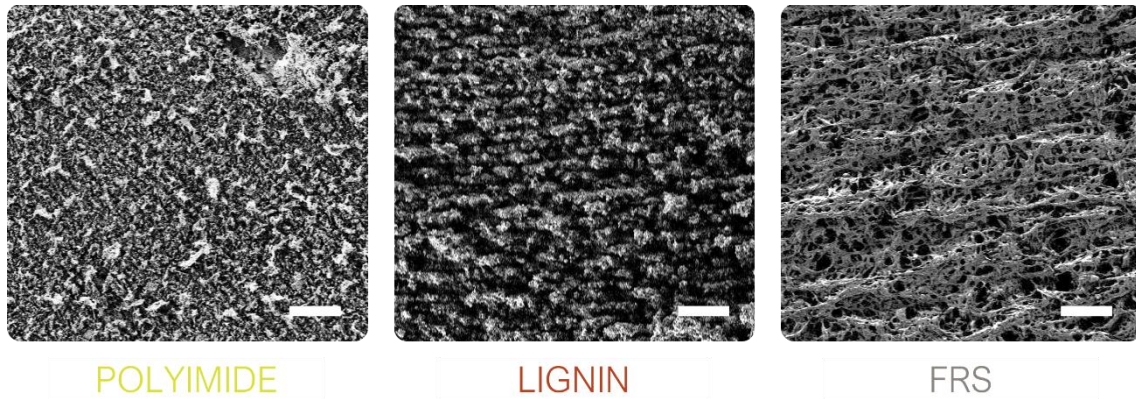
Figure S6: SEM images of LIG surface engraved over the polyimide, lignin coating over cardboard and Flame Retardant Spray (FRS) over cardboard. Scale bar: 100 \mu\text{m} .
