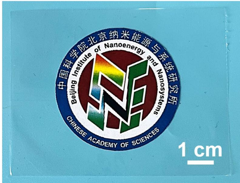
**Fig. S3** The optical image of P(VDF-TrFE-CFE) film.
