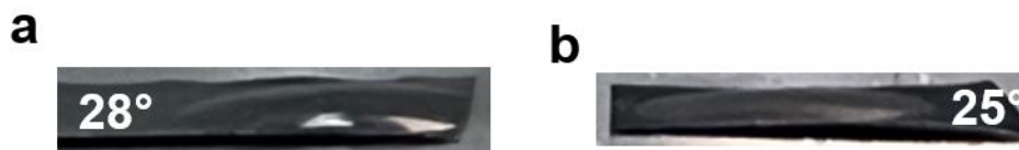
Figure S15. Optical images showing a single droplet of the carbonate electrolyte on the surface of (a)94@H0 electrode (b)94@H10 electrode.
