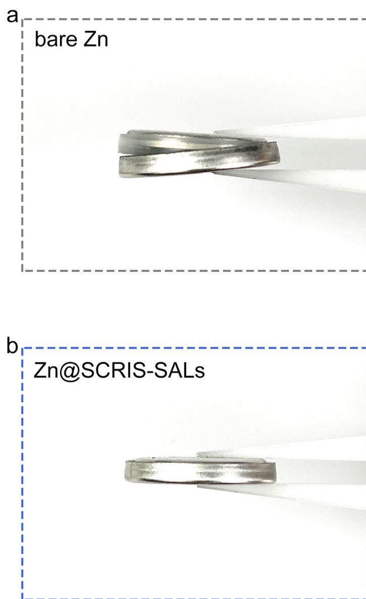
Fig. S11 The photograph of (a) bare Zn and (b) Zn@SCRIS-SALs symmetric cells under a high areal capacity of 20 \text{ mAh cm}^{-2} at a high current density of 10 \text{ mA cm}^{-2} after 5 cycles.
