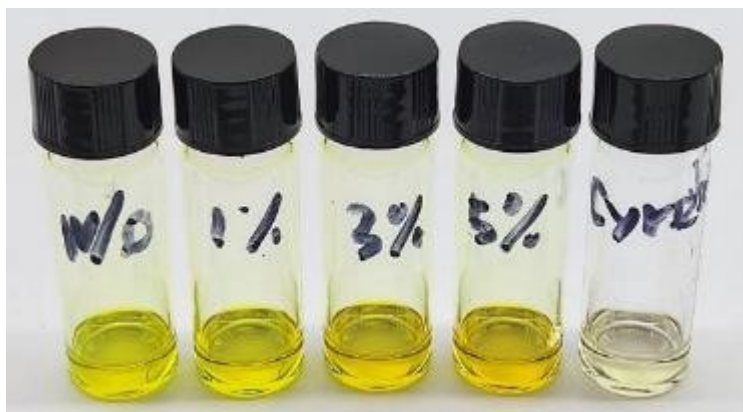
Fig. S11. The photograph of \text{PbI}_2 solutions with different content of Cyrene (without, with 1%, 3% and 5%) and Cyrene solution.
