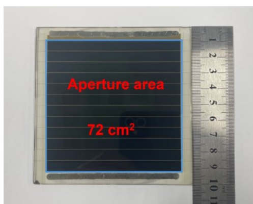
Fig. S23. Large-area module images. By employing a process similar to that of small-area modules and through careful design, we have successfully fabricated large-area modules with an efficiency of 21.91%. The only difference from the small-area modules lies in the width of the sub-cells.
