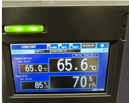
Figure S17. Damp-heat testing equipment operating at 65°C and 85% relative humidity.
