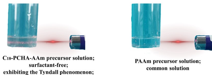
Fig. S1 Illustration of Tyndall phenomenon in C_{18} -PCHA-AAm and PAAm precursor solutions.
