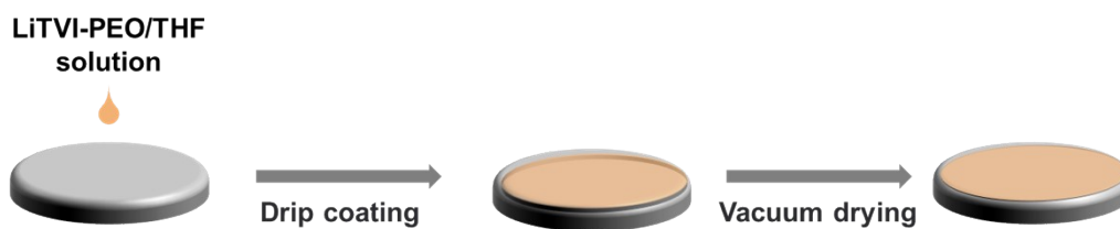
Fig. S24: Schematic illustration of drop-casting method to prepare HAcI@Li electrode.
