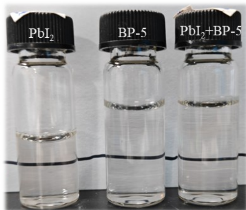
Figure S12. The pictures of different kinds of aqueous solutions. The clear black line indicates that there is no insoluble complex formed between BP-5 and lead iodide.
