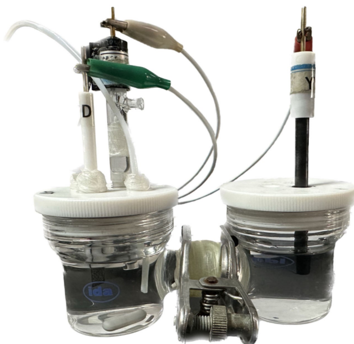
Figure S4. The optical photograph of the H-cell system for urea electrosynthesis testing.
