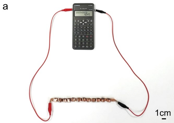
Fig. S36 a) Photograph of a commercial calculator operated by 12 CCA-MEG units in a series connection. b) Photograph of a commercial thermo-hygrometer operated using 5 CCA-MEG units in series connection.
