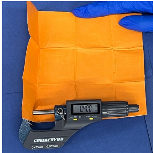
Figure S16. Encapsulated flexible Zn||C-PVA/PAN|| NH 4 V 4 O 10 with thickness of 400 \mu\text{m} .
