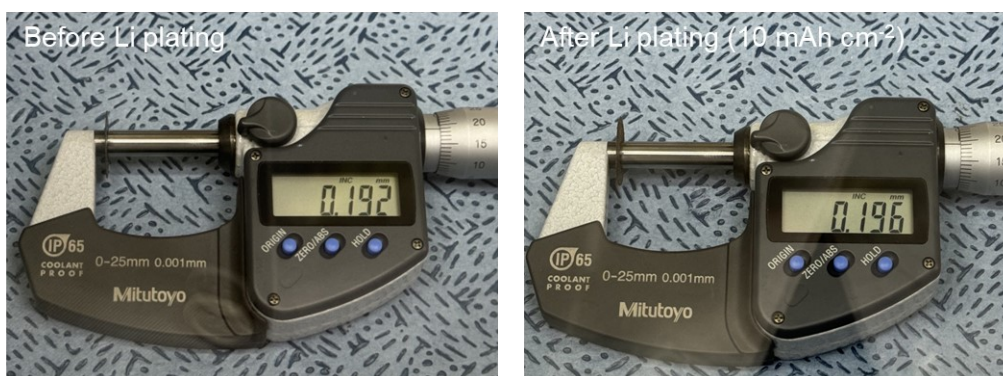
Fig. S28. Thickness measurements of the Janus film anode substrate before and after Li plating, captured using a thickness measurement device. A difference of 0.004 \mu\text{m} is considered to be within the measurement error. Hence, the thickness of the film remains virtually unchanged after Li plating, confirming the complete accommodation of Li within the CF film
