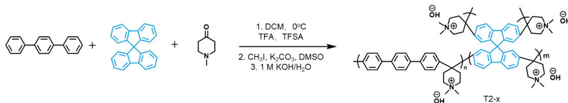
Scheme S3. Synthesis route of T2-x. Note: the x of T2-x refers to the theoretical molar percentage of Sp/(Sp+biphenyl) in the polymer.
