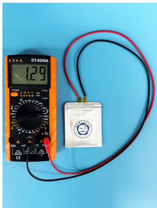
Fig. S35 Optical picture of the ZC-8-2-50@Zn||NVO pouch cell before bent and pierced examinations.
