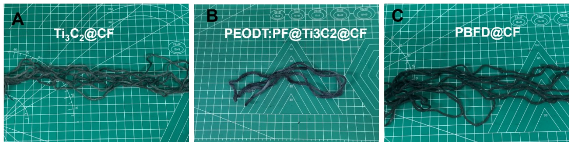
Fig. S2 | (A) \text{Ti}_3\text{C}_2 @CFs fibers. (B) PEDOT:PF@ \text{Ti}_3\text{C}_2 @CFs fibers. (C) PBFD@CFs fibers.
