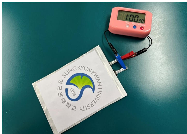
Fig. S45 Zn||MnVO pouch cell-powered electronic alarm clock.
