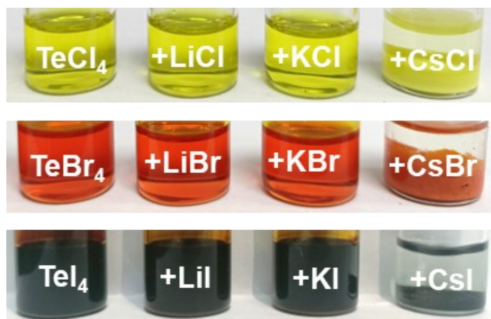
Figure S8. Visualization experiments of the reaction between \text{TeX}_4 and AX salts.
