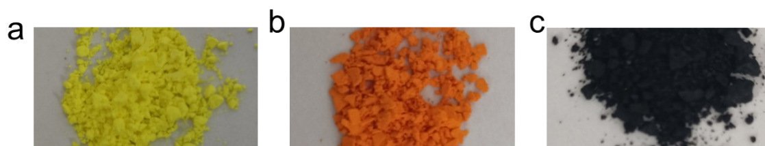
Figure S9. The solid products obtained by adding different CsX in Figure S5 (a) CsCl; (b)CsBr; (c) CsI.
