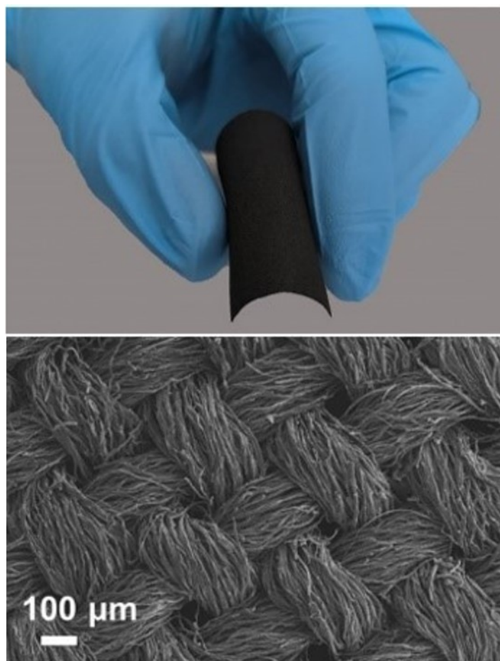
Figure S1. (a) Optical photograph of NCFC showing its good flexibility. (b) SEM image showing the woven fiber-like structure of NCFC.
