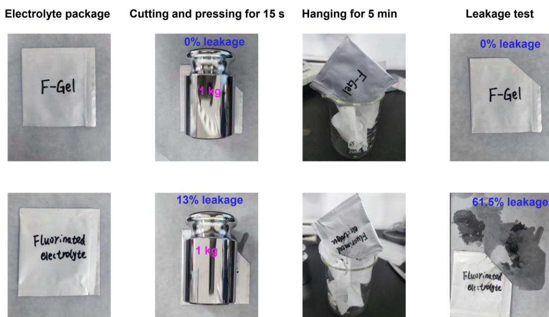
Fig. S11 Leakage tests of F-Gel (upper panels) and 1 M LiPF 6 in EA-2F: FEC fluorinated electrolyte (lower panels).
