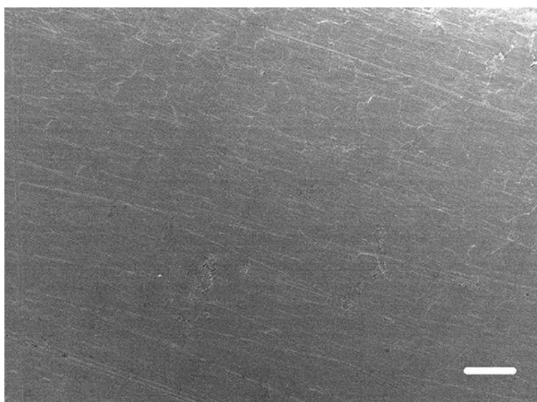
Figure S17 SEM image of fresh Zn foil (scale bar: 10 \mu\text{m} ).
