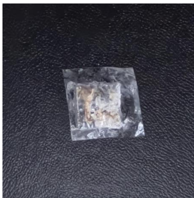
Fig. S6. Photo of Ca-deposited Aquivion cation exchange membrane after 44 h electrolysis.
