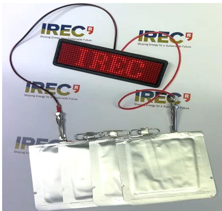
Fig. S47 Four series-connected pouch-battery cells powering a light board.
