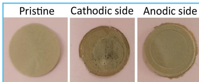
Fig. S12 PBI separators before and after pre-activation.
