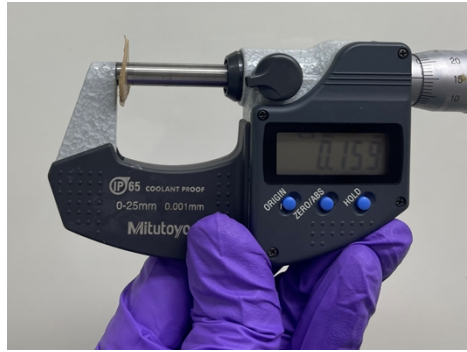
Fig. S6 Thickness measurement of the PBI electrolyte.
