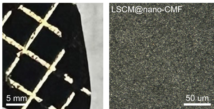
Figure S10. Digital images of the LSCM@nano-CMF fuel electrode subjected to Raman mapping after stability test for CO 2 electrolysis at 800 °C.
