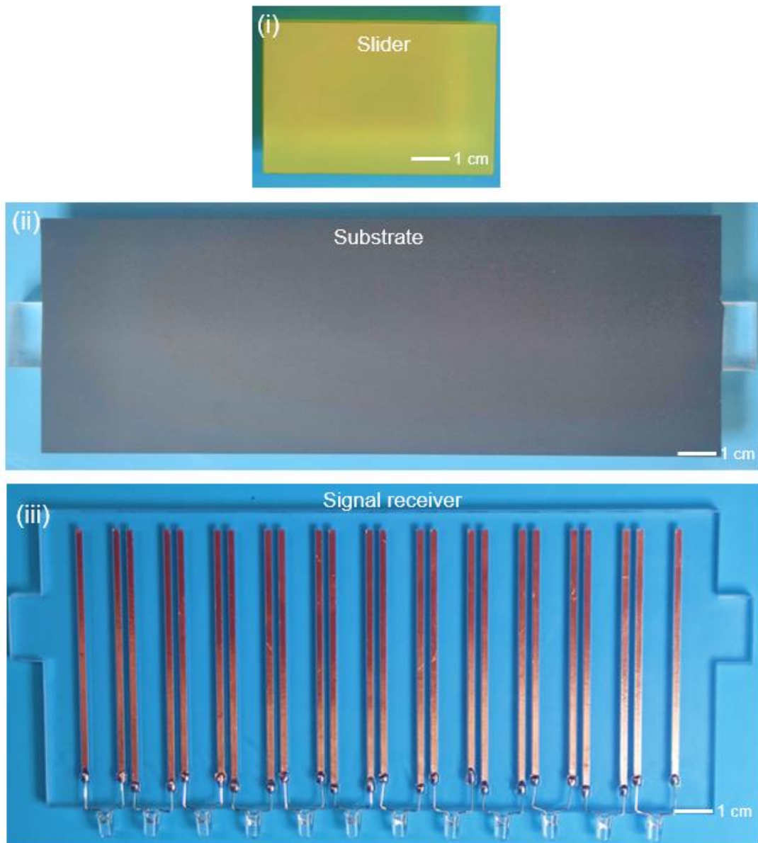
Figure S19. The construction of the visual wireless position sensing system. (i) Digital photograph of the slider. (ii) Digital photograph of the substrate. (iii) Digital photograph of the signal receiver.
