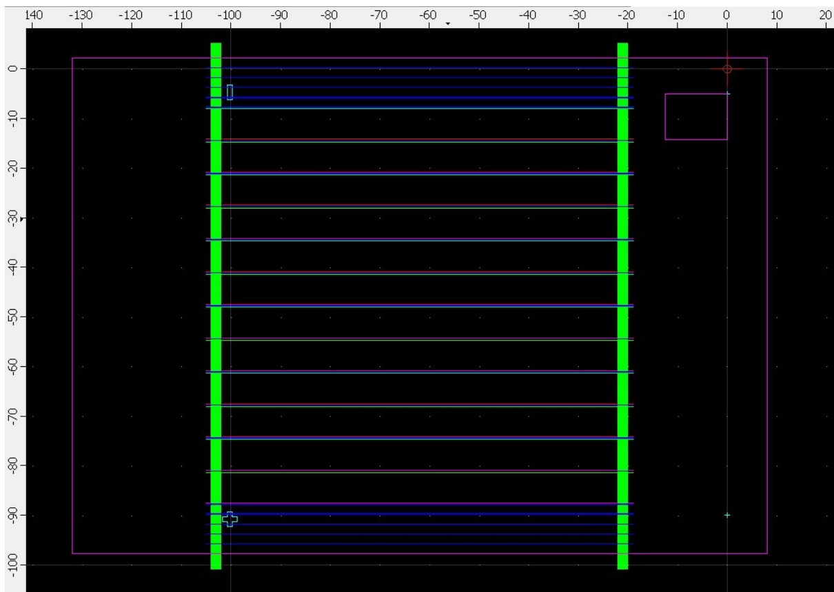
Figure S2: Schematic layout of the module for modules area of < 64\text{cm}^2 . The module consists of 12 individual cells connected in a series. The total area of the individual cells within the modules is around 4.93\text{ cm}^2 . This translates to a total active area of around 59.2\text{ cm}^2 whereas the total area of the module including bus bars and electrical interconnection area stands at 64\text{ cm}^2 . a) Red lines indicate P1 laser scribes, b) Blue lines indicate P2 laser scribes and c) Green lines indicate P3 laser scribes.
