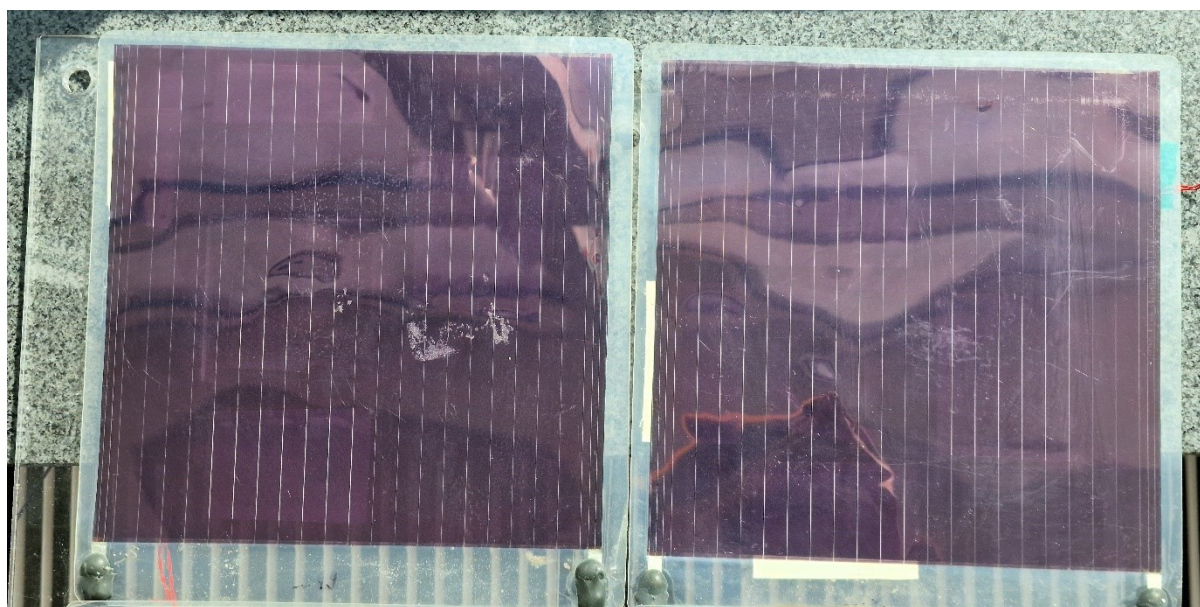
Figure S13: Visual inspection of the modules OPV 45° (left) and OPV 90° (right) after outdoor exposure.
