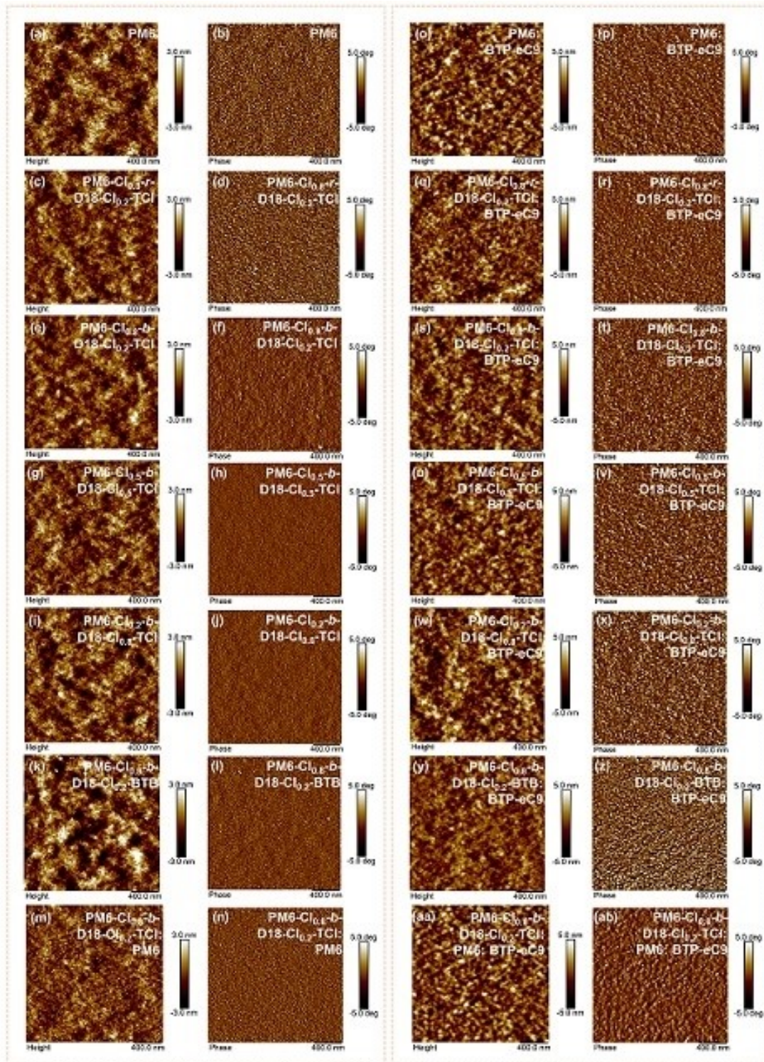
Figure S25. AFM characterization of high figures ( 2 \times 2 \mu\text{m} ) and phase figures ( 2 \times 2 \mu\text{m} ) of pristine MCD films PM6 (a, b), PM6-Cl 0.8 -r-D18-Cl 0.2 -TCl (c, d), PM6-Cl 0.8 -b-D18-Cl 0.2 -TCl (e, f), PM6-Cl 0.5 -b-D18-Cl 0.5 -TCl (g, h), PM6-Cl 0.2 -b-D18-Cl 0.8 -TCl (i, j), PM6-Cl 0.8 -b-D18-Cl 0.2 -BTB (k, l), and PM6-Cl 0.8 -b-D18-Cl 0.2 -TCl: PM6 (m, n) as well as corresponding MCD: BTP-eC9 blend films PM6: BTP-eC9 (o, p), PM6-Cl 0.8 -r-D18-Cl 0.2 -TCl: BTP-eC9
