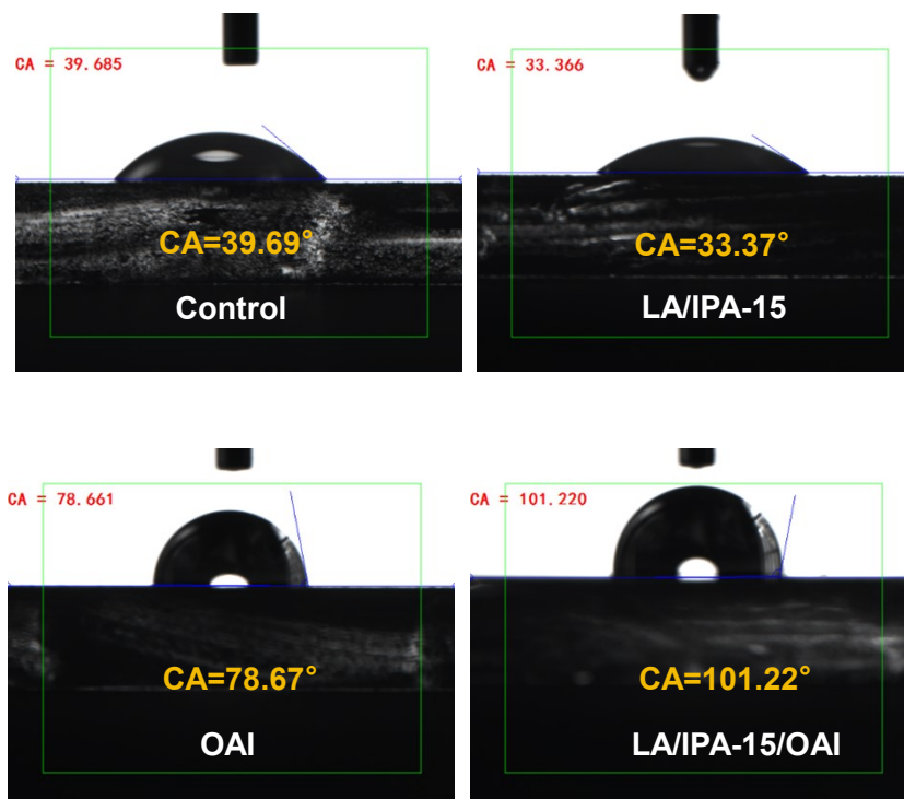
Figure S9. Water contact angle (CA) of perovskite films with different treatments.
