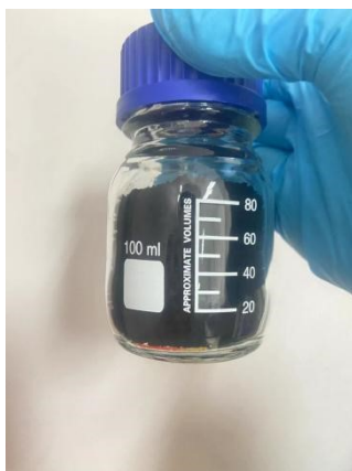
Fig. S1 \text{FeTe}_2/\text{CN} was generated in situ on a larger scale using high-purity tellurium powder.
