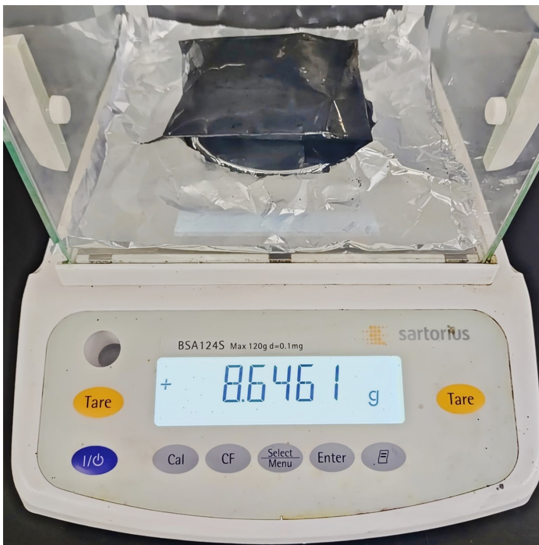
Fig. S18. Photograph of the AuPd@C catalyst obtained in the scale-up production. The raw material of single synthesis includes 1.0 g of \text{HAuCl}_4 \cdot 3\text{H}_2\text{O} , 0.5 g of \text{PdCl}_2 and 7.95 g of Ketjen black (carbon support).
