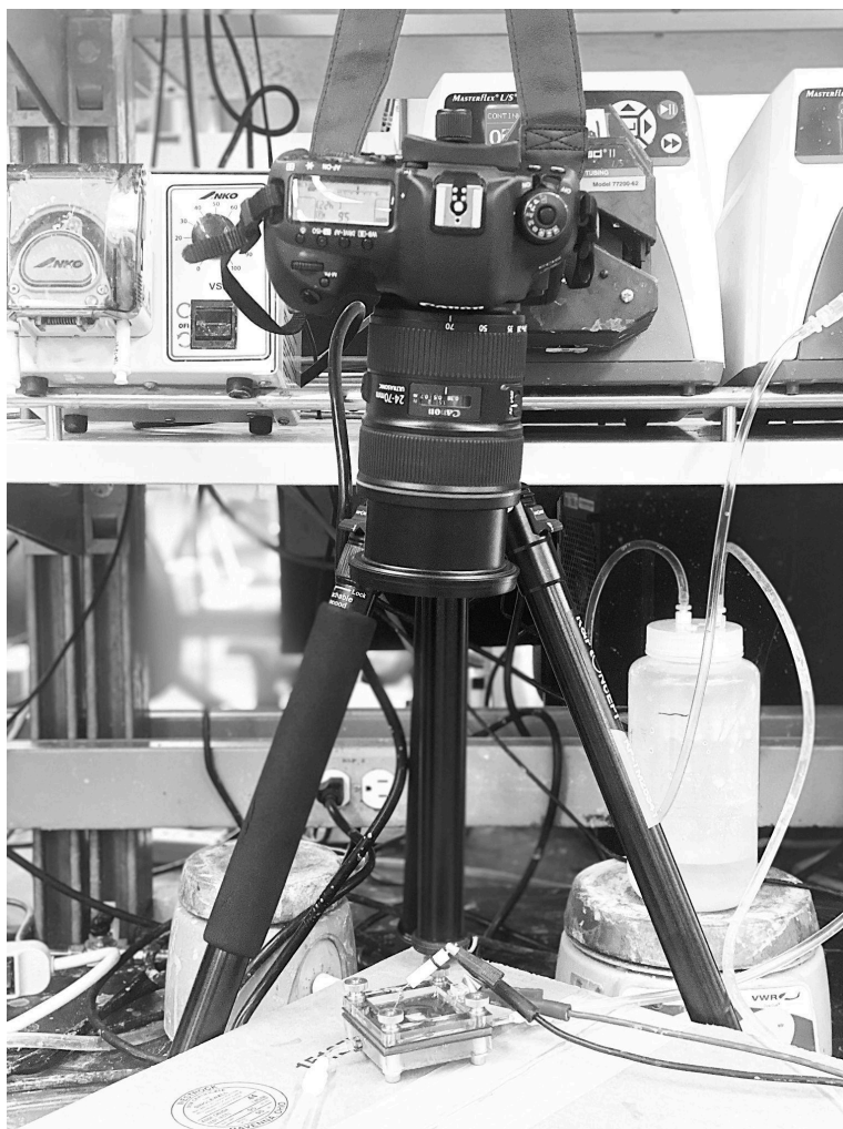
Figure S13. The optical photo of the operando imaging system. The imaging system consisted of a modified two-compartment electrolyser with an open cathode compartment so we could image the CEM through the transparent catholyte with a high-resolution single-lens reflex (SLR) camera fixed above the electrolyser.
