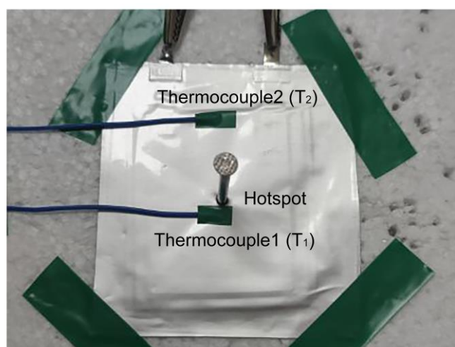
Fig. S12 Physical display of the needle penetration test. The thermoregulating capability of TCC is expected to effectively delay battery temperature rise, especially in dealing with local hot spots.
